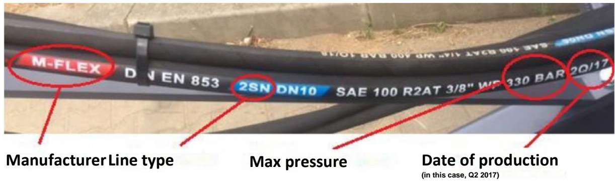
Figure 20. Marking of the hydraulic lines
