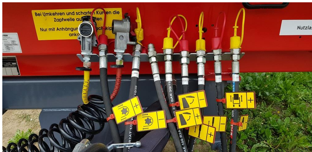
Figure 21. Pictograms on the hydraulic connectors for easier connection to the tractor
